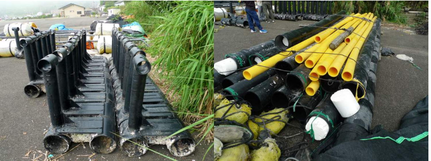
Cage damaged by cargo ship. Undamaged components are extracted to be reused.
