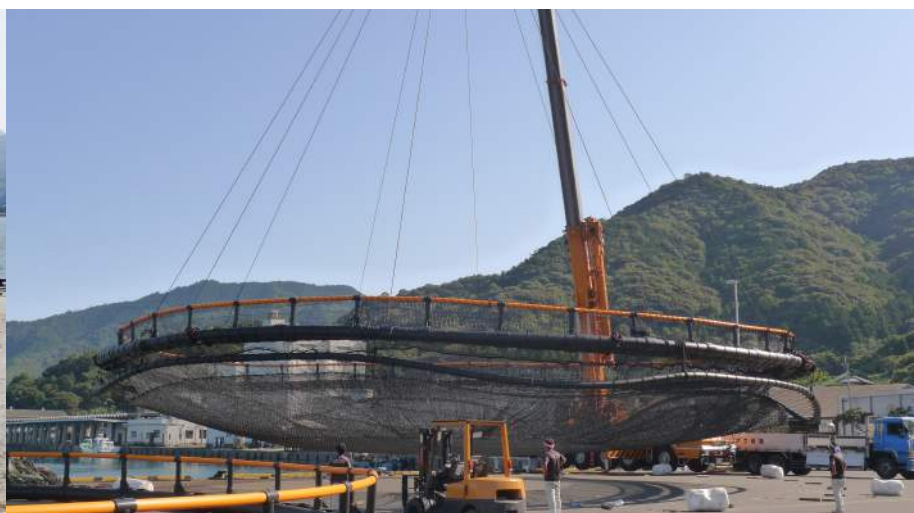
355m cage with KikkoNet and sinker tube
