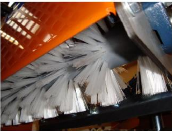
Cover plate of the brush has been shortened on the underside with 25mm. Also the mounting plate of the bearing block has been shortened on the underside.
