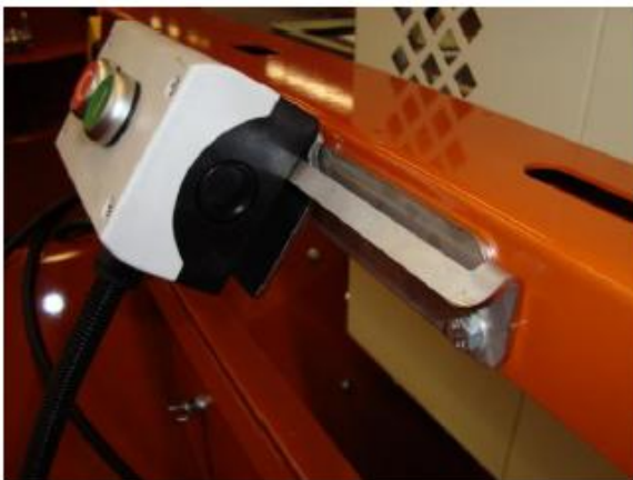
Assembly bracket for the control box.
