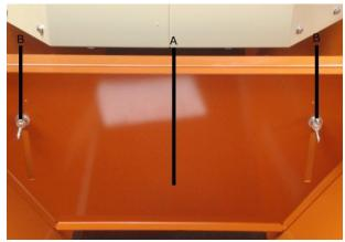
The height of the soil plate (A) in the soil bin can be adjusted to set the amount of potting soil reaching the elevator.
