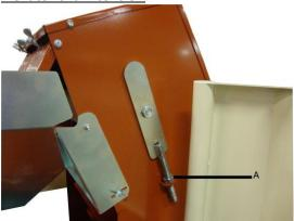
The elevator chain tension is correct when it can move  $\pm$  20 mm in the centre.
