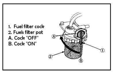
Figure 6.3 | The fuel filter
