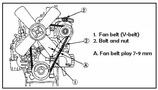
Figure 6.9 | Tighten the V-belt
