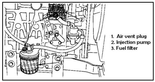
Figure 6.4 | Fuel filter in engine block
