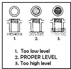
Figure 6.8 | The level of battery acid
