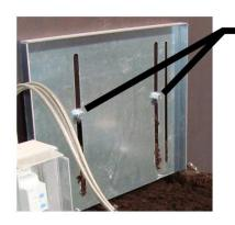
The soil slide controls the amount of soil on the subsequent conveyor belts.
