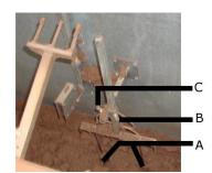
There are two soil level sensors (A) behind the fluffers in the bunker belt.
