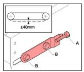
The tension is correct when the belt hangs down ± 40mm in the centre.
